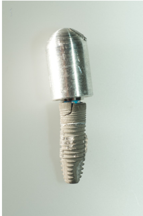
Fig. 6 Fracture of the implant body
