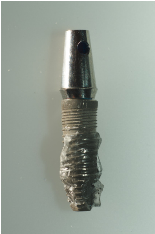
Fig. 5 Plastic deformation of the Implant body and the Abutment
