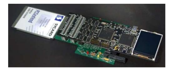
CAM Inspector probe plugs on top of a standard Syscard extender (included with the probe). Level translation buffer isolate captured signals on the bus and feed them into a FPGA containing capture logic. Capture traces are then fed to a 32 bits CPU that can either :
